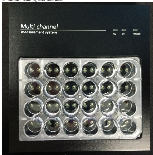
Figure 1. The real time O 2 and pH measurement system with 24-well microplate
